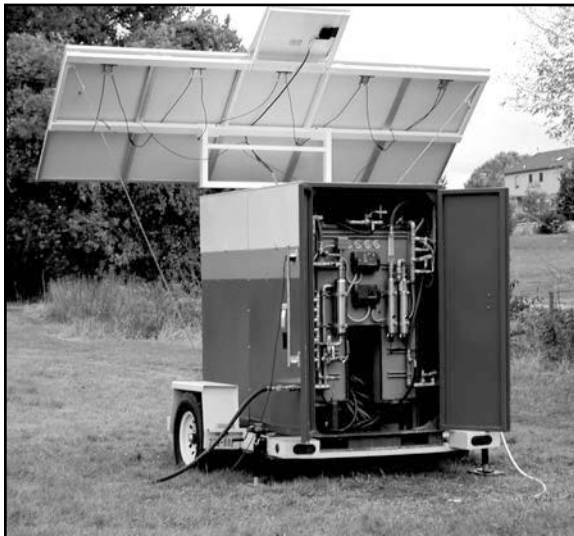
IWC's trailered water purification unit: Finally, a deployable system which does not depend on diesel, or filters, or chemicals. The unit can stand alone in the field for years without spares, and pump out up to 30,000 US gallons a day of potable water. It was designed to be fully "soldier-proof" and can generate additional electricity to power sat-phones or laptops.
