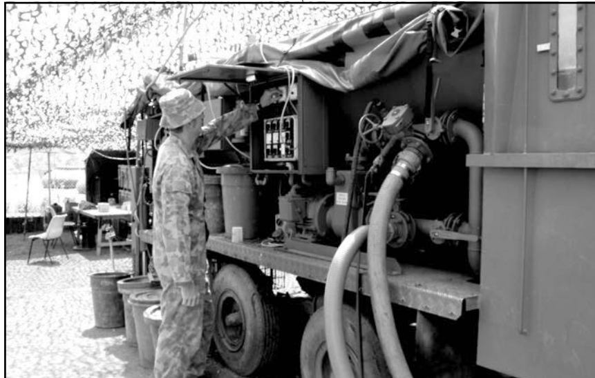
The hard way: An Australian Army sapper from the 3rd Combat Engineer Regt. operates a truck-mounted water purification unit in Afghanistan. Earlier-generation water purification plants have depended heavily on diesel power, chemicals, and regular filter changes, adding to the logistical burden in deployment and sustained operations. They have not been designed as relatively maintenance-free “leave behind” units which could bolster civil-military relations and minimize the need for external support for remote villagers.
